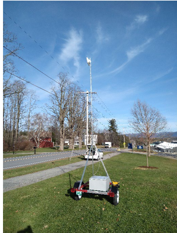
Figure 8 The mobile traffic monitoring platform
