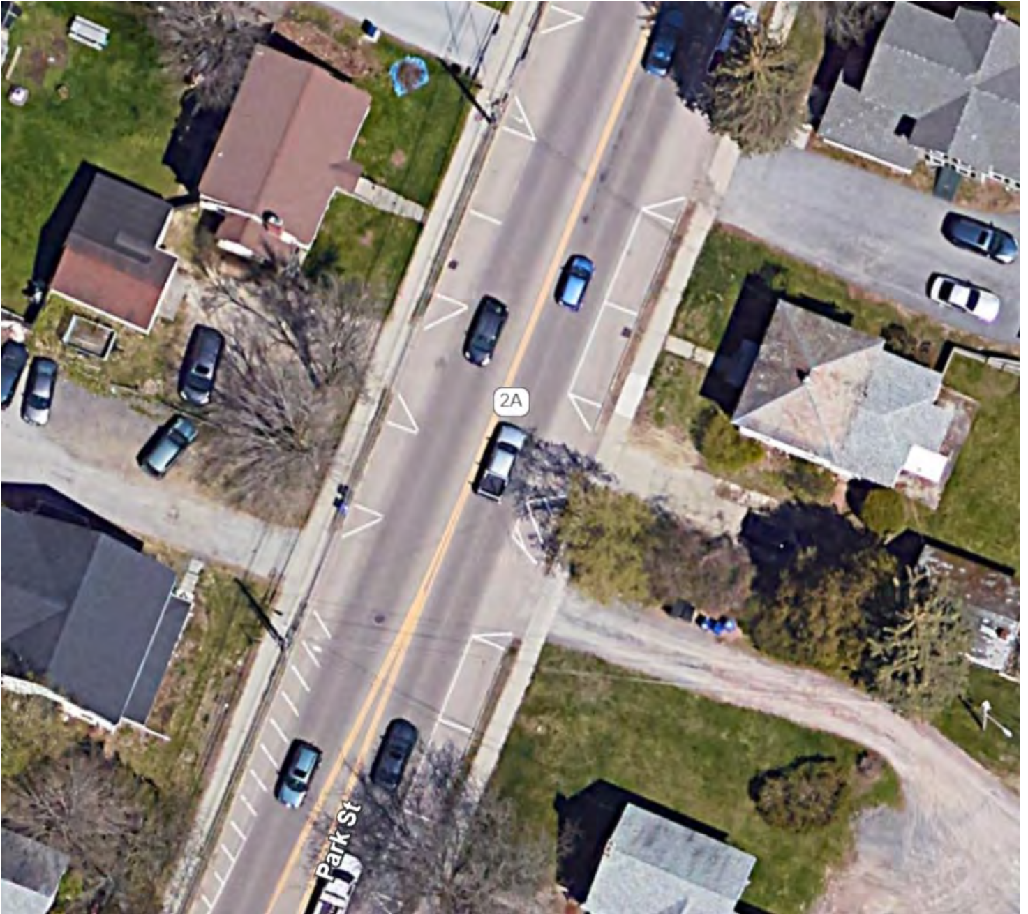
Figure 2: Example of striping existing conditions on Park Street between Franklin Street and Silver Bow Terrace. Note the empty parallel parking on both sides of the street and no accommodation for bicycles.
