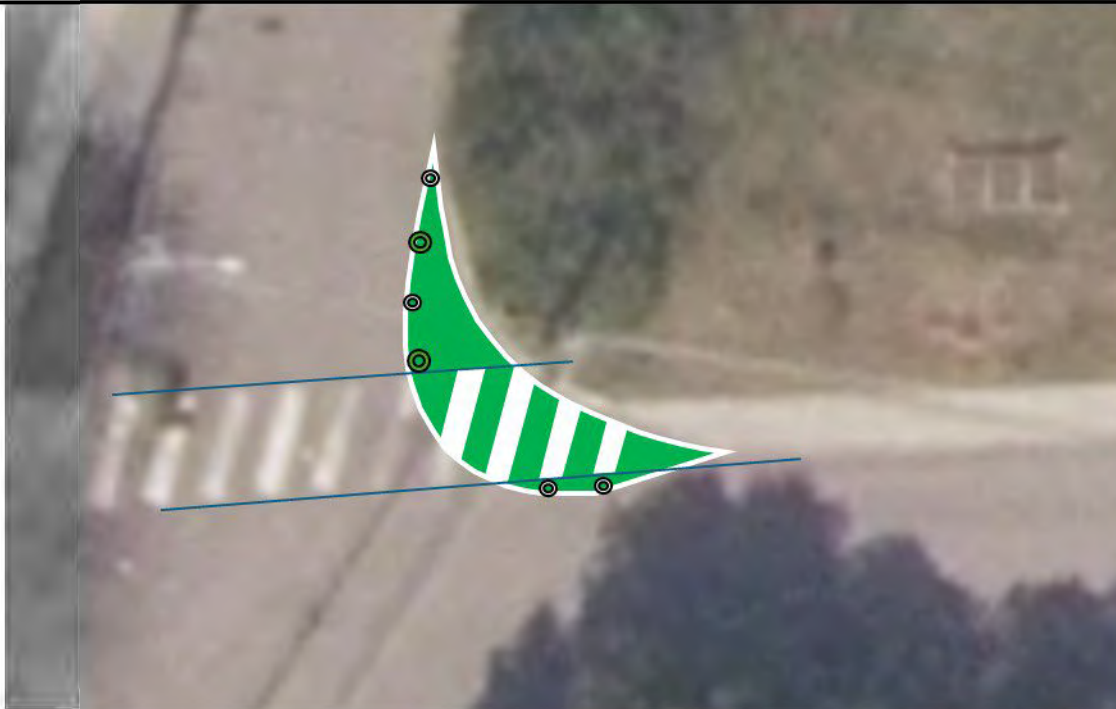
Figure 7: Option 2's proposed curb radius reduction with painting and installation plan. Stop bar to be repainted in existing location, eight flexi-posts to be installed at locations marked by circles, and 15-foot curb radius to be painted in white as shown
