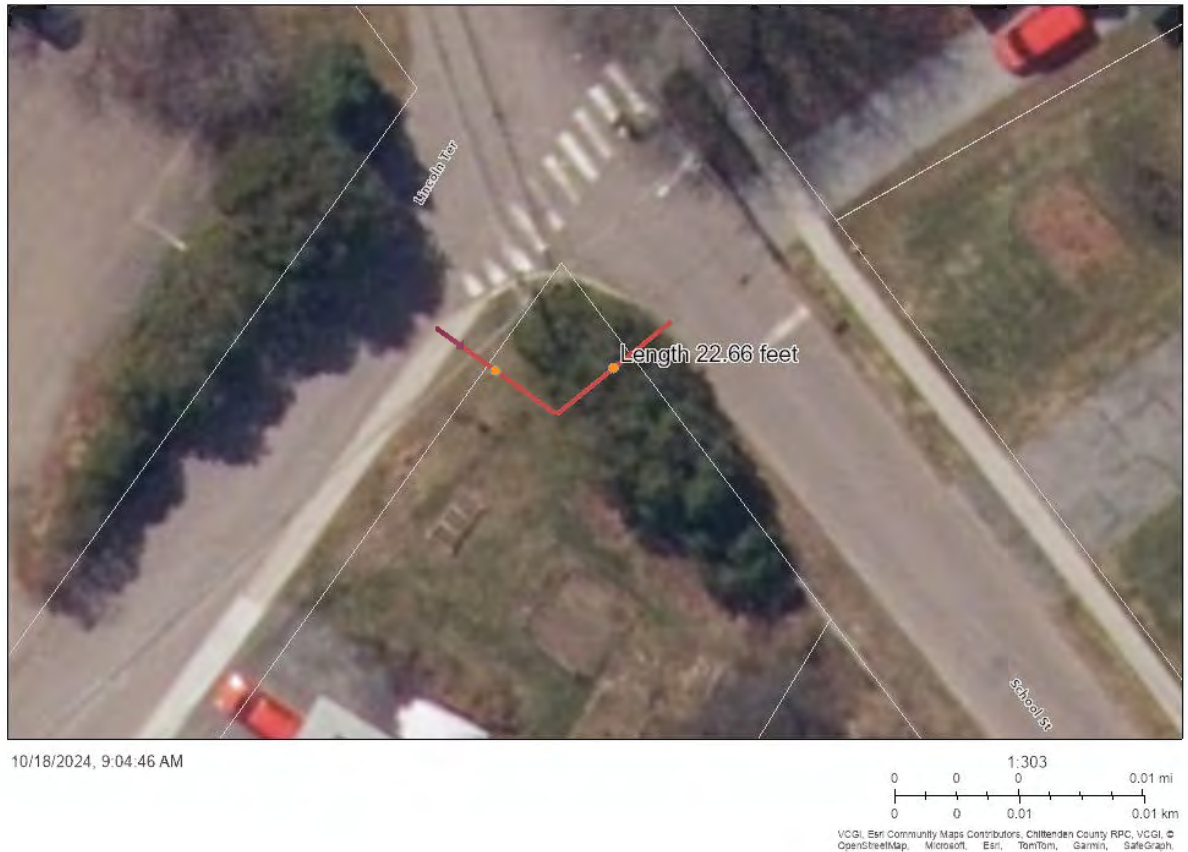
Figure 1: Aerial view of existing conditions at Lincoln Terrace and School Street with the curb radius measured in red. Source: Vermont Center for Geographic Information (VCGI)
